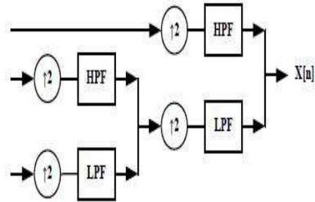
Figure 3. Wavelet reconstruction process.
