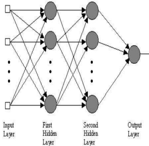
Figure 5. MLP architecture with two hidden layers [34].
