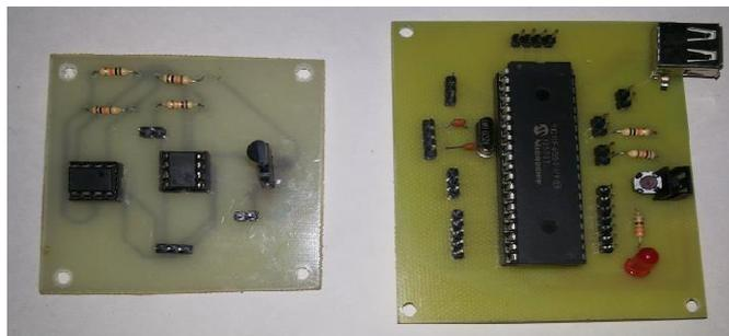
Fig 4. LM35 circuit with amplifier and PIC board
