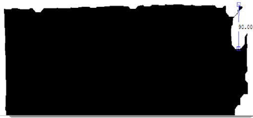
Fig. 10. Wear measurement using imtool function in MATLAB
