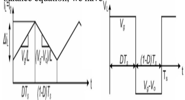
Fig (7.a) Inductor current waveform
