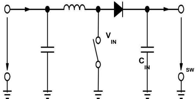
**Fig 8 Boost Converter Power Stage.**
