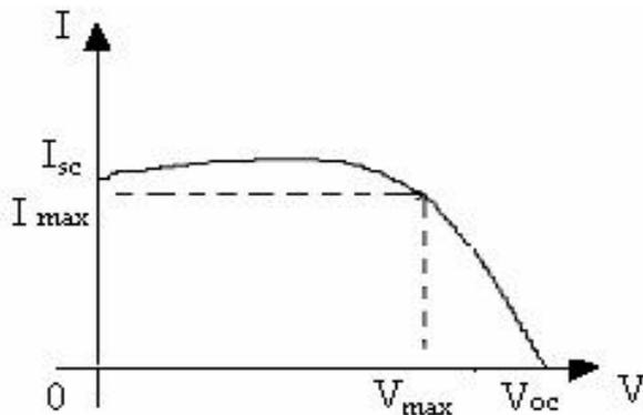
Fig. 3(a) VI Characteristics in PV Cell.
