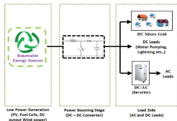
**Fig. 1. Typical renewable energy system with DC-DC converter.**
