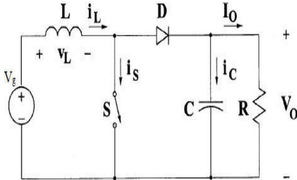
Fig 4 Circuit diagram of boost converter.
