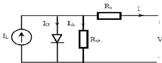
**Fig.2. Diode principle circuit.**
