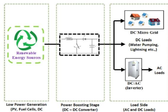
**Fig. 1. Typical renewable energy system with DC-DC converter.**
