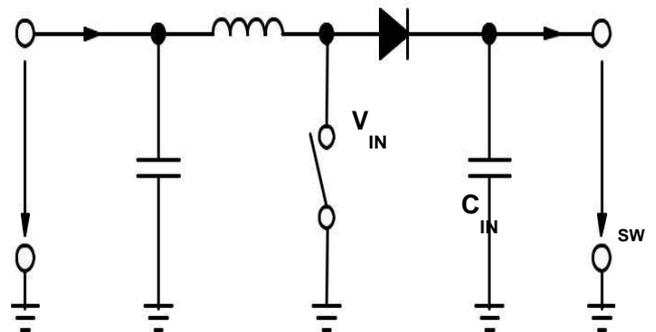
**Fig 8 Boost Converter Power Stage.**
