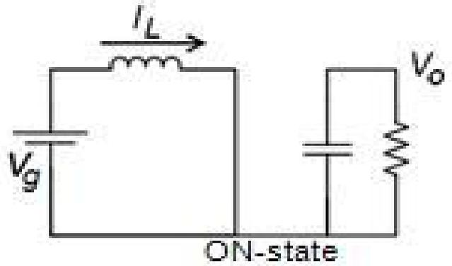
Fig (6) the ON state diagram of the boost converter.
