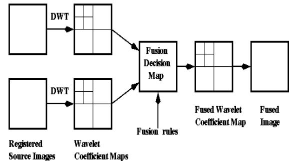
**Fig.1: Processing stage of Image fusion system**
