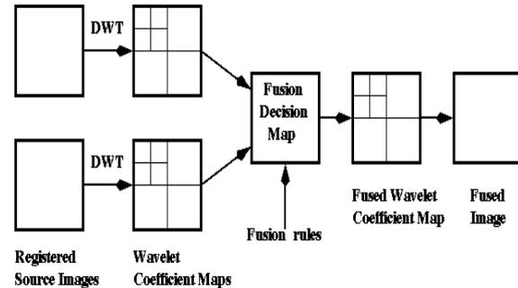
**Fig.1: Processing stage of Image fusion system**
