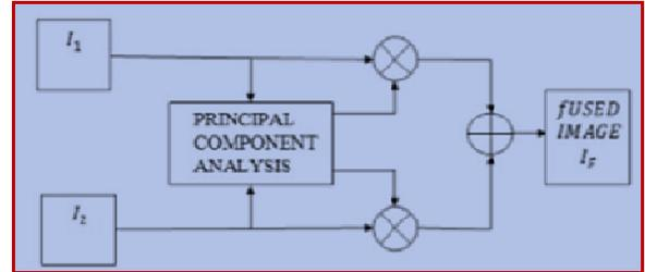
**Fig.2: Information flow diagram in image fusion scheme employing PCA**
