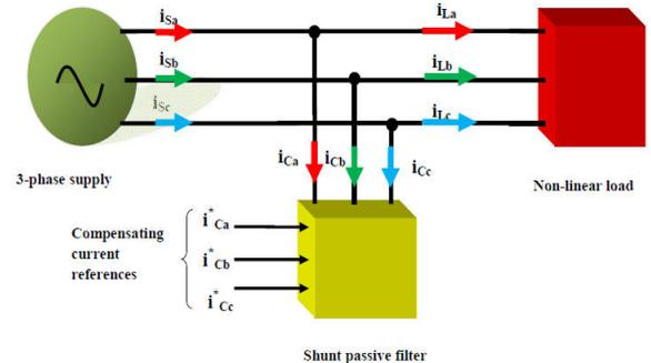
**Fig1. Passive Filter**
