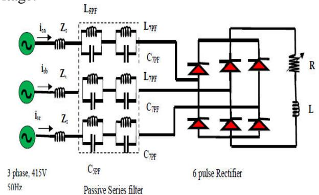
**Fig.2. Schematic diagram of a ac-dc converter with R-L load and passive series filter at input**
