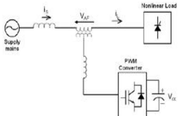
**Fig. 4 Principle configuration of a VSI based series active power filter**
