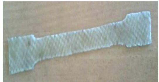
Fig. 5. Specimen for tensile test
