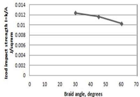
Fig. 9. (b). Variation in izod impact strength with braid angle
