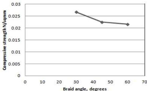
Fig. 19. (b). Variation in compressive strength with braid angle.
