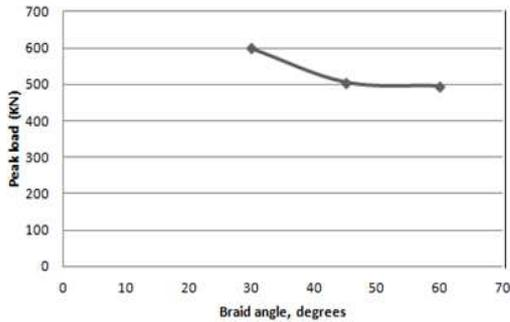
Fig. 10. (a). Variation in peak load with braid angle.
