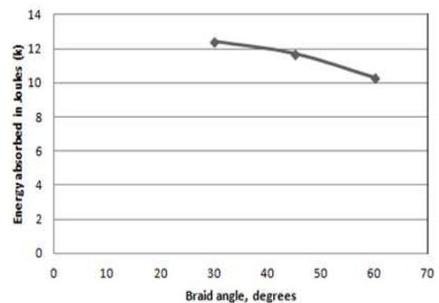
Fig. 9. (a). Variation in impact energy absorbed with braid angle.
