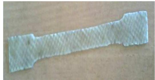
Fig. 5. Specimen for tensile test
