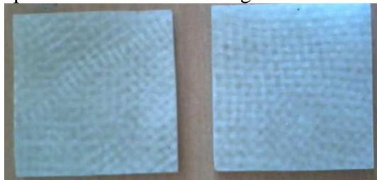
Fig. 4. E-glass braided composite specimen
