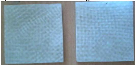
Fig. 4. E-glass braided composite specimen
