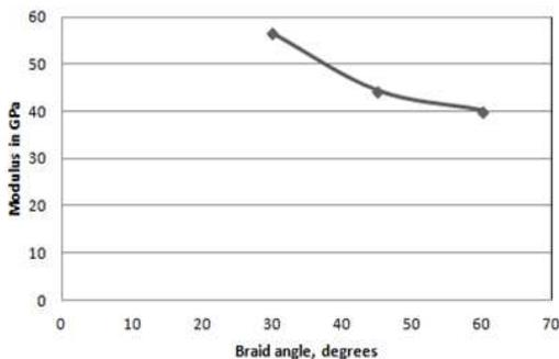
Fig. 8. Variation in modulus with braid angle.
