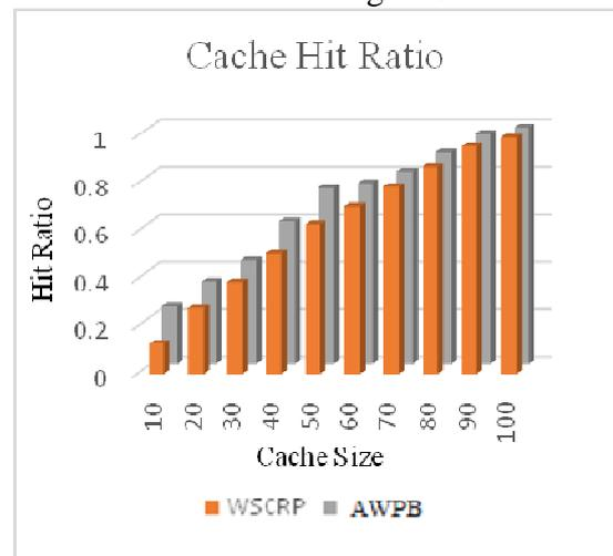
**Figure 5: Cache Hit Ratio Comparison**
