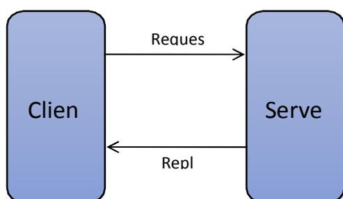
Figure 1: Client Server Architecture
