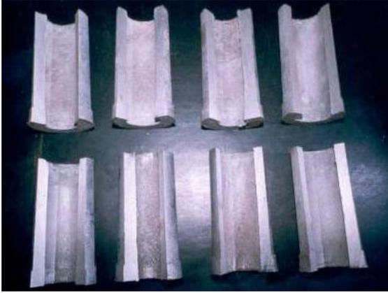
**Fig. 1 Specimen by Centrifugal Casting**
