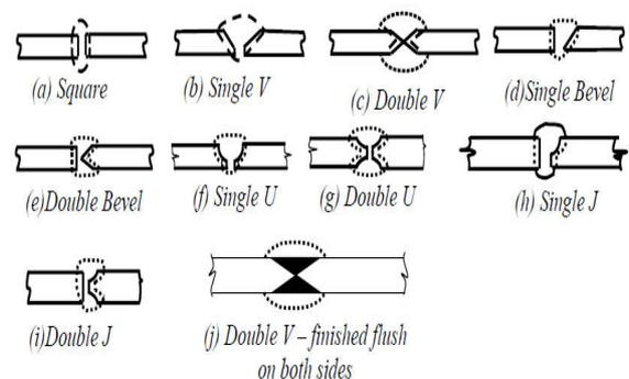
**Fig 2 Butt Joints**
