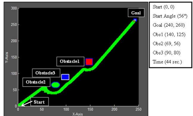
**Fig. 7. Trajectory of the singlemobile robot with 3 obstacles**
