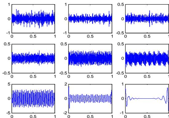
Fig.3 8Level DWT of vibration signal for healthy motor at full load
