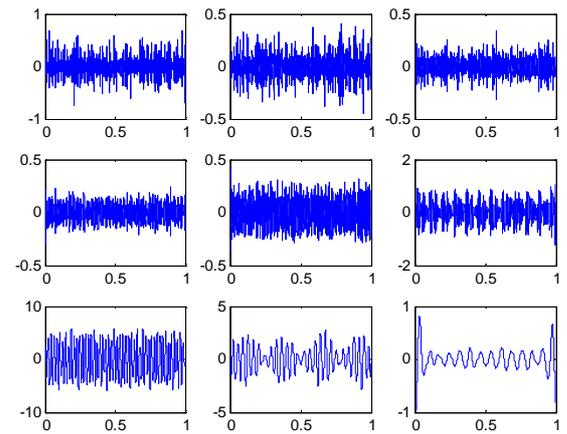
Fig.4 8 Level DWT of vibration signal for faulty motor at full load
