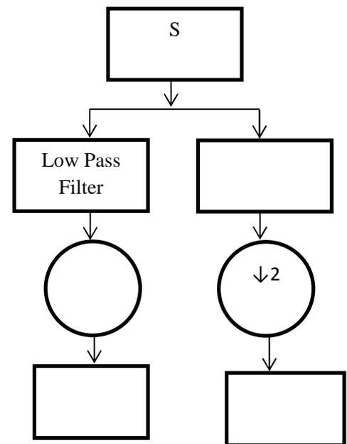
Fig.1 DWT decomposition of a signal
