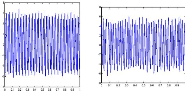
Fig.2 Vibration signal under full load for healthy and faulty motor respectively
