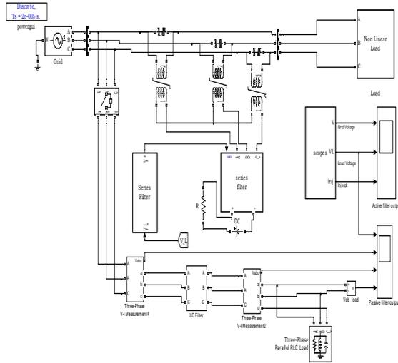
**Fig.1:** A simulink model of THD analysis for the improvement of power quality in three phase AC system by using active passive filter.
