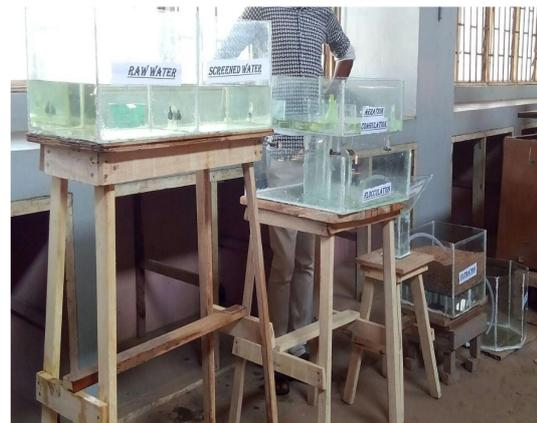
Plate 2.0 Side View of the Treatment Plant Model.
