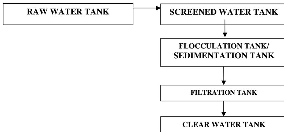
Fig. 2. Schematic Diagram of the Water Treatment Plant Model.
