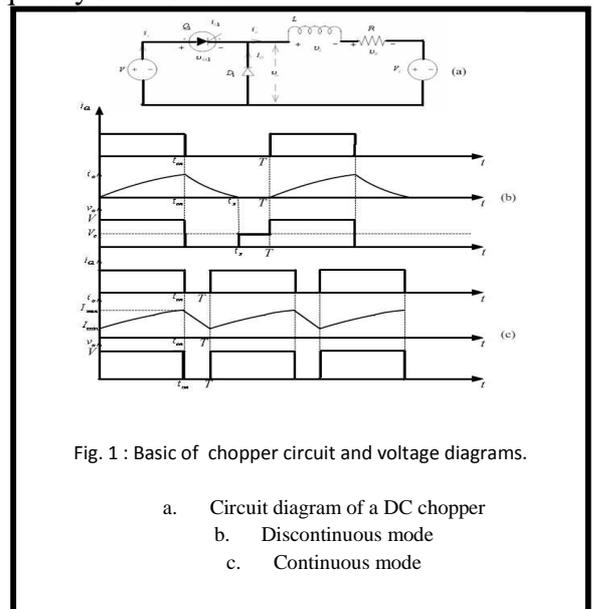
Fig. 1 : Basic of chopper circuit and voltage diagrams.
