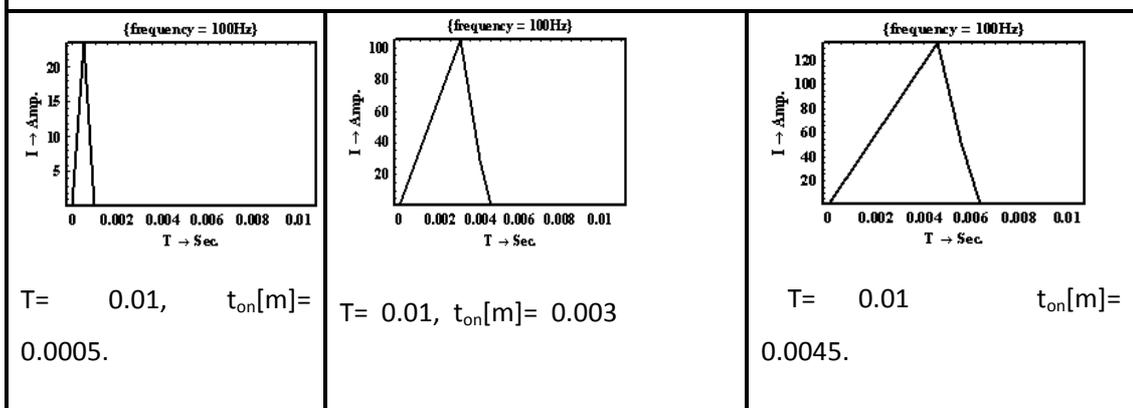
Fig. 10: Relationship between I and T at voltage batteries ( $V_B$ )= 60
