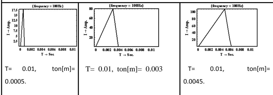
Fig. 11: Relationship between I and T at voltage batteries ( $V_B$ )= 72
