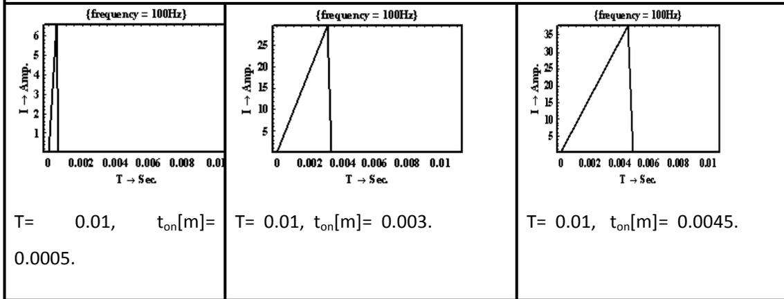
Fig. 13: Relationship between I and T at voltage batteries ( $V_B$ )= 96
