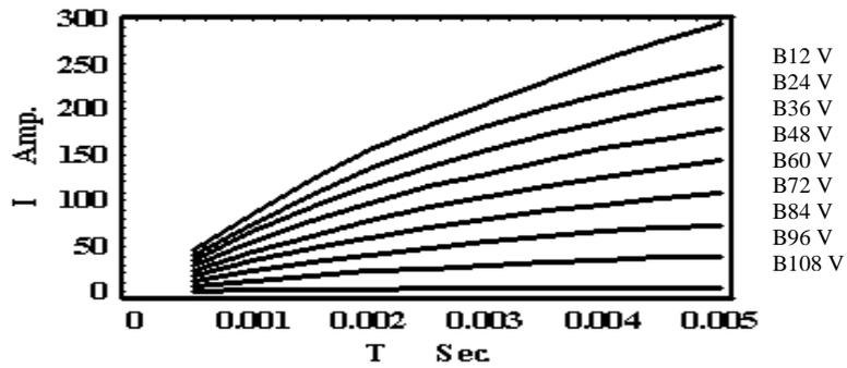
Fig. 16: The relationship between ( $I_{max}$  &  $t_{on}$ ),  $V_{inj}$  (battery) takes as a parameter.
