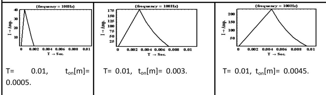
Fig. 7: Relationship between I and T at voltage batteries ( $V_B$ )= 24
