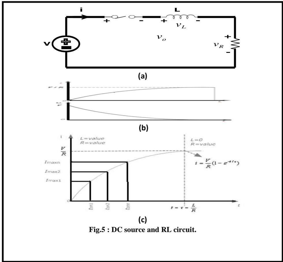
Fig.5 : DC source and RL circuit.
