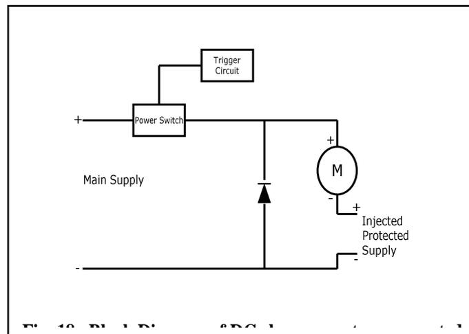
Fig. 18: Block diagram of the proposed DC chopper system
