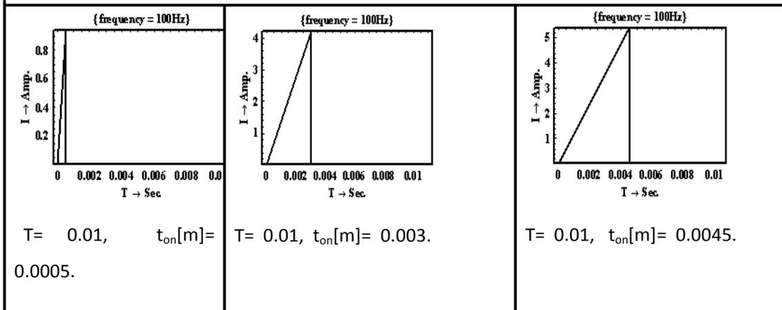
Fig. 14: Relationship between I and T at voltage batteries ( $V_B$ )= 108
