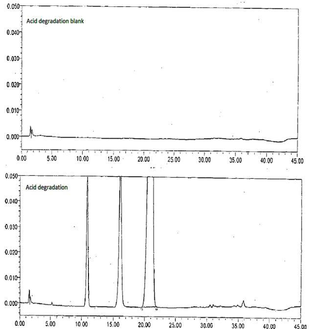
Figure 5: Acid degradation and diluent blank
