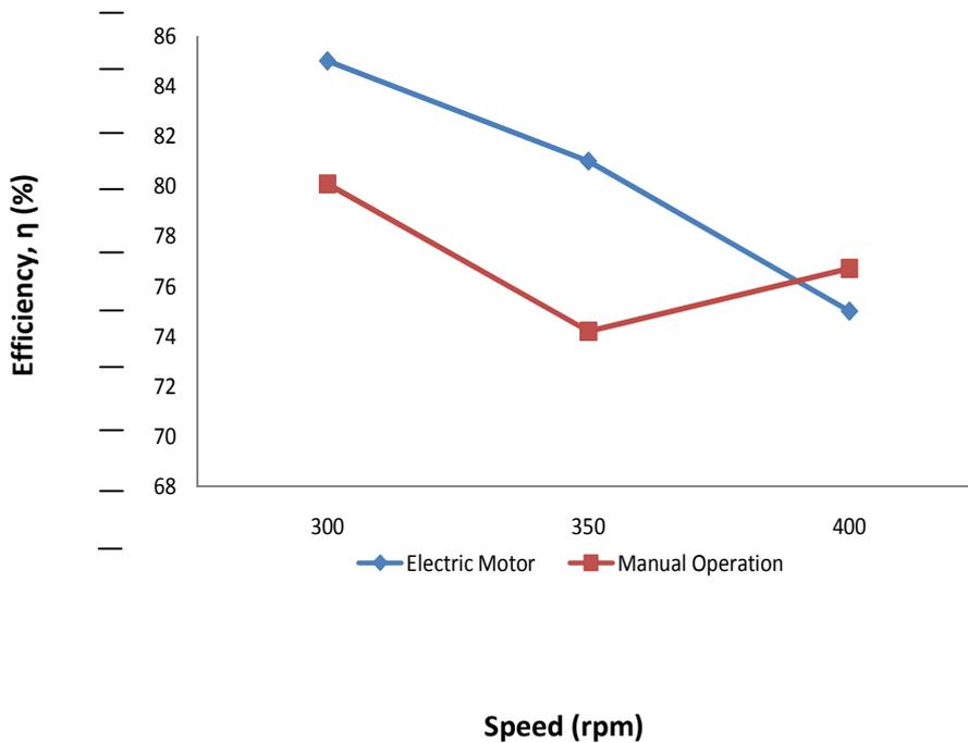
**Figure 4:** Effect of speed on Cassava Chipping Efficiency
