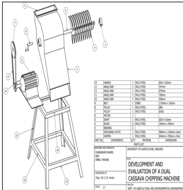
Figure 1: Exploded view of cassava chipping machine
