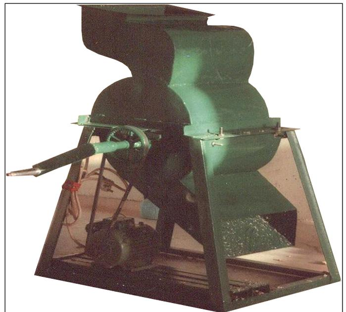
Figure 2: Assembled Cassava Chipping Machine (to show components, a safety guard in belt drive has been removed).
