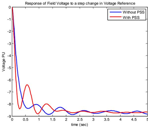
Figure 6.2 Response of IEEE 50 machine system
