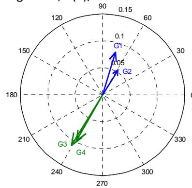
Figure 5.8 Compass Plot for 2-Area, 4- Machine System
