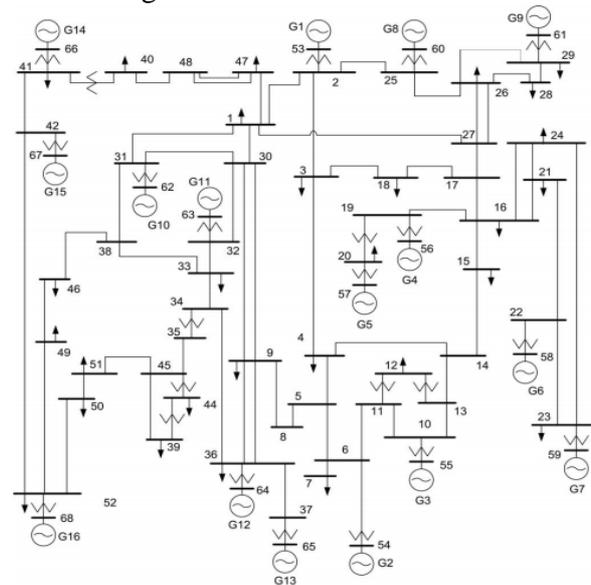
Figure 5.1 Single line Diagram of 16 machine 68 bus test system
