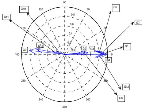
Figure 5.2 Compass Plot for 16 Machine System
