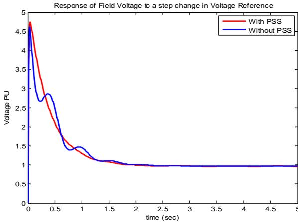
Figure 6.1 Response of NPCC 16 machine 68 bus system
