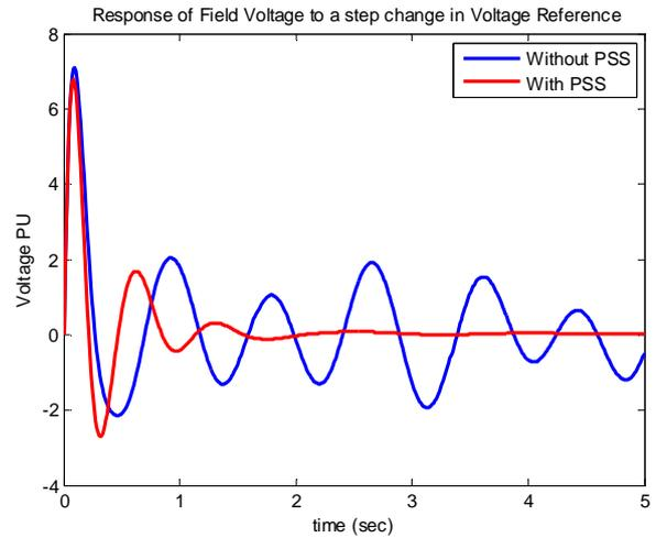
Fig. 6.4 Response of Kundur's Two Area Four Machine System
