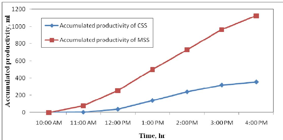
Fig.5. Variation of accumulated productivity of MSS and CSS w.r.t. time
