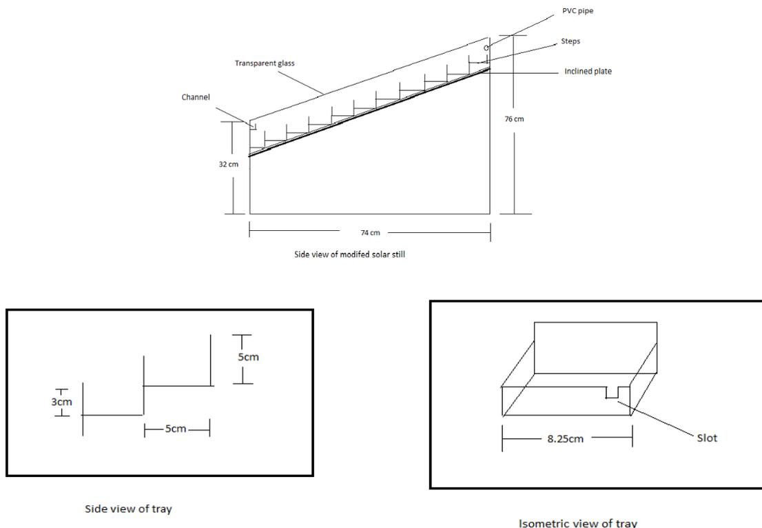
Fig. 1 Schematic diagram of modified solar still
