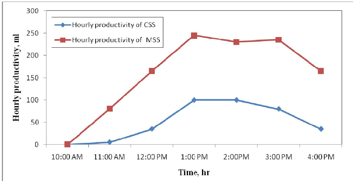
Fig.4. Variation of hourly productivity of MSS and CSS w.r.t. time
