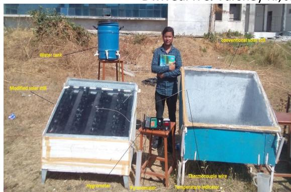
Fig.2. Experimental setup of conventional and modified solar still with instruments
