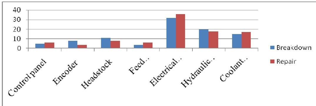
Fig. 1 CNC Lathe machine sub-system failure frequency and Downtime
