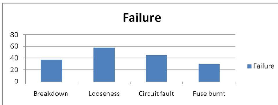
Fig 2 Failure Mode of CNC Lathe
