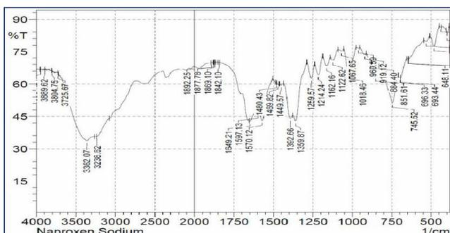
Figure No: 2 FTIR of Naproxen Sodium Soft Gelatin capsules
