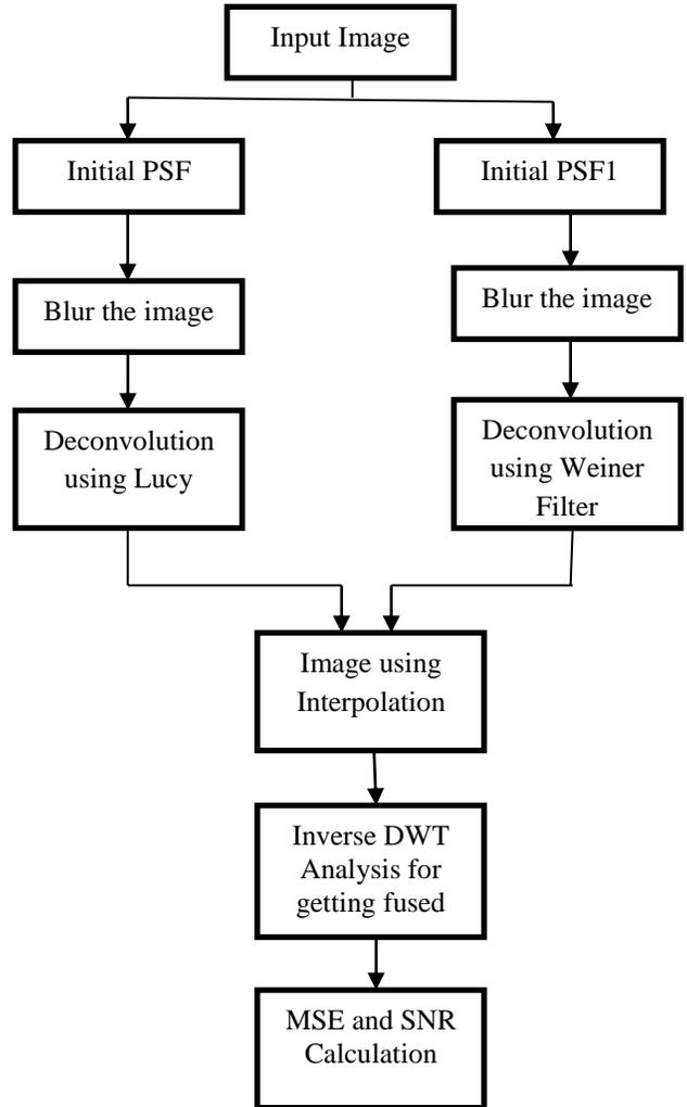
Fig 4: Image restoration interpolation flow chart for image restoration using Lucy Richardson with Wiener Filter
