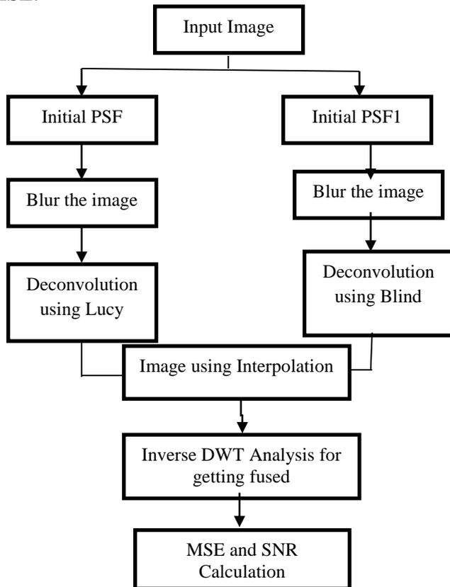
Fig.3: Image restoration using interpolation Lucy Richardson with Blind Deconvolution
