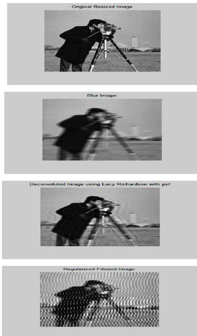
Fig. 9(a) original image (b) blur image (c) deconvoluted image using L-R with PSF (d) Regularized filtered image
