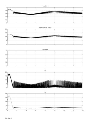
Fig 4: Mechanical, Electrical Torque and rotor speed with pitch angle
