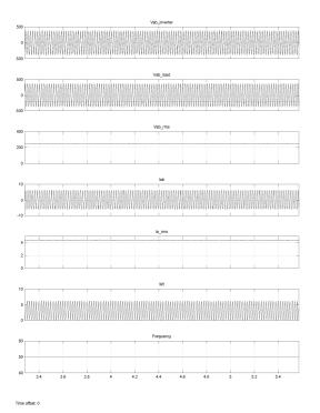
Fig 6: Load voltage and current RMS values
