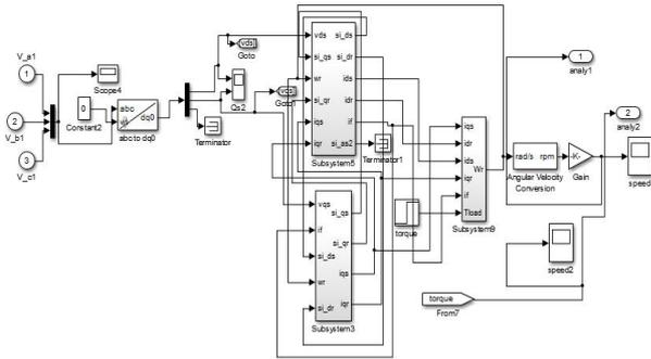
**Fig 4 Shows the Mathematical Model of Induction Motor**
