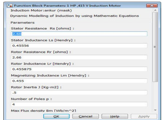
**Fig 8 Induction motor and its parameters**
