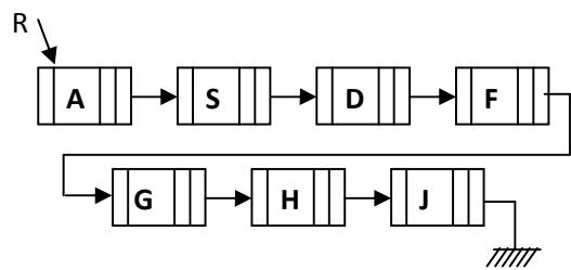
Figure 3.1.1: Creation of Link List with Sequence of the Data in Inorder
