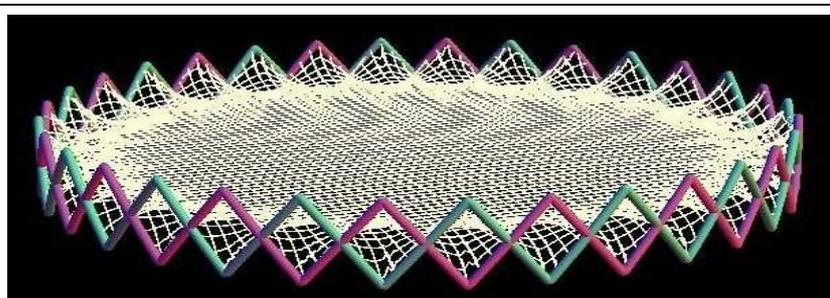
**Fig. 1 – The supporting structure for the solar reflector**
