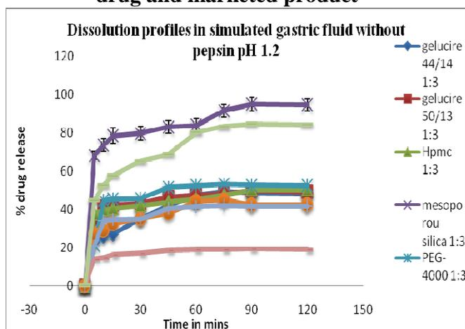
**Fig 6** Dissolution profile of the different solid dispersion (1:3) carriers along with the plain drug and marketed product
