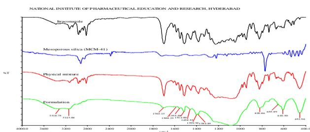
**Fig 2: FTIR Spectroscopy of Itraconazole, mesoporous silica, physical mixture, formulation**
