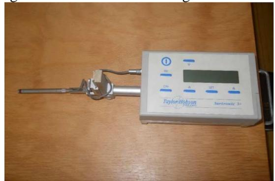
Figure 1. Surface roughness tester
