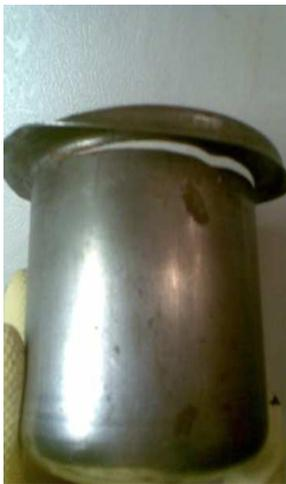
**Figure 4. Blanks with Cracks**
