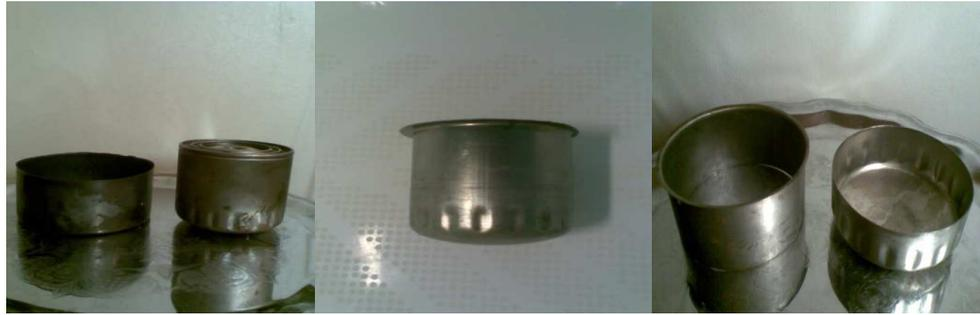
**Figure 6. Filter Casing Blanks Produced with New Method**
