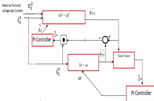
Fig.2 Model Reference Adaptive System (MRAS) structure for parallel estimation of rotor speed and stator resistance
