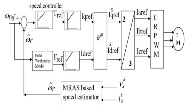
Fig. 3 Indirect field oriented control structure of IM for parallel estimation of rotor speed and stator resistance
