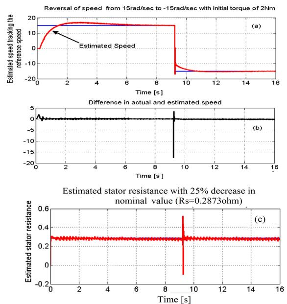
Fi Fig.4. Step change in reference speed from 15rad/sec to -15rad/sec at 9 seconds and initial load torque of 2 Nm with 25%
