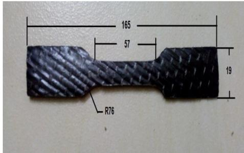
Figure 2: Sample Piece for Tensile Test
