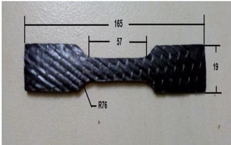
Figure 2: Sample Piece for Tensile Test
