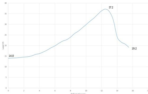
Figure3:Load vs Deformation Graph
