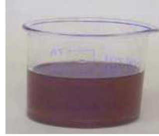
Fig 2. Oil expelled from karanja seed
