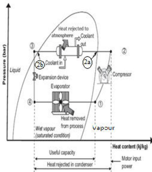
**Fig. 1.** Single-stage refrigeration cycle.
