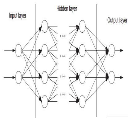
Fig 2. Multi-layer feed forward network [3]
