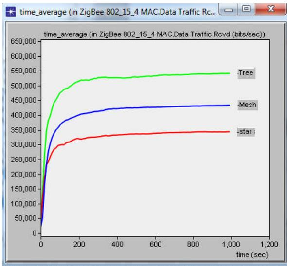
Figure 4: MAC. Data Traffic Received (bits/sec)
