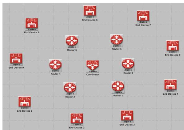
Figure 1: Network Structure for Star, Mesh and Cluster Tree Topologies
