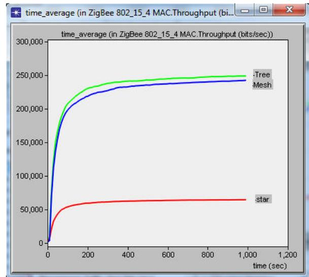
Figure 2: Throughput (bits/sec)
