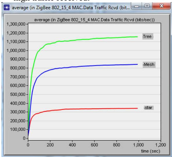
Figure 7: MAC. Data Traffic Received (bits/sec)
