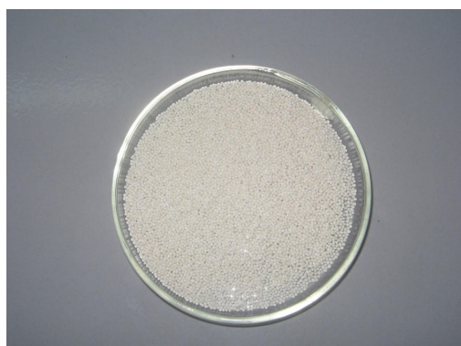
Figure 1: Pellets obtained by process of extrusion spheronizer
