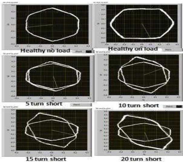
**Figure 1:** plots of Id and Iq for various condition under load and no load condition
