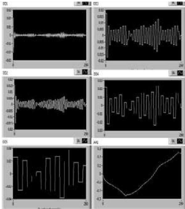
**Figure 4:** Detailed and approximate level coefficients level of  $I_q$  for healthy system.
