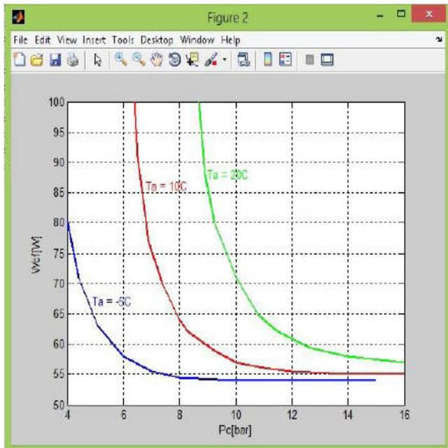
**Fig.5. Condenser Fan power & Condenser Pressure**
