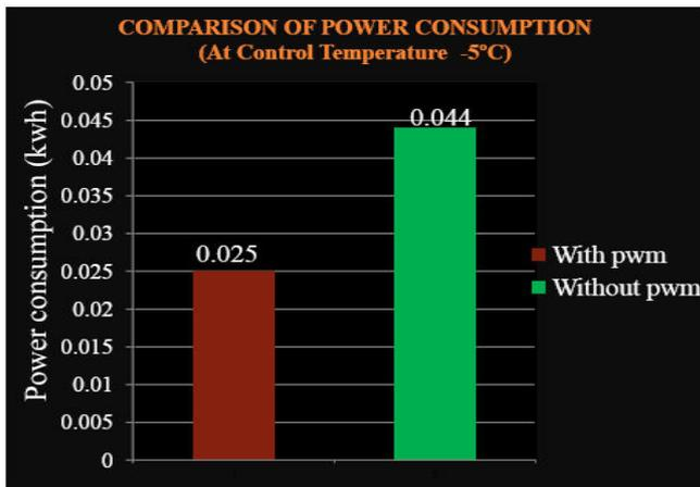
3. Comparison of power consumption with and without pulse width modulation technique at control temperature -25<sup>0</sup>C.
