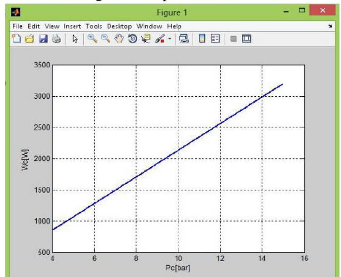
**Fig.4. Compressor Power & Condenser Pressure**
