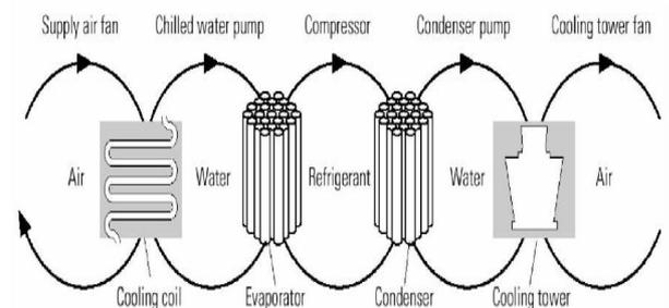
**Fig.3. Heat Transfer Loop in Refrigeration System**
