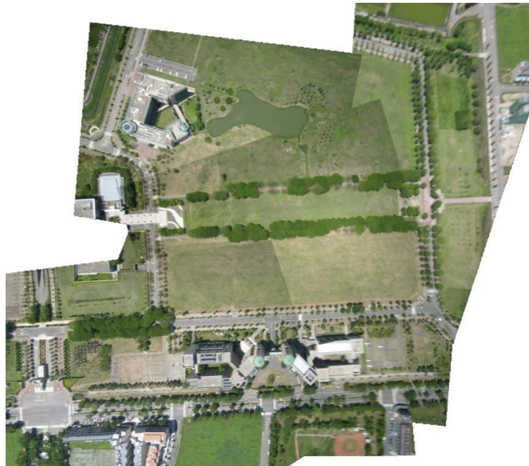
Fig. 4: The corrected, edited and mapinterlinking photo from camera installed in UAV
