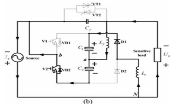
Fig. 4. Operating conditions during negative half-cycle.(a) V1 switched on. (b) V1 switched off.
