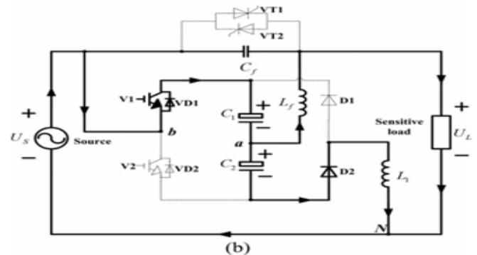
Fig.3. Operating conditions during positive half-cycle. (a) V2 switched on.(b) V2 switched off.
