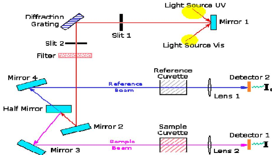
**Figure 1. Scheme diagram of the spectram**
