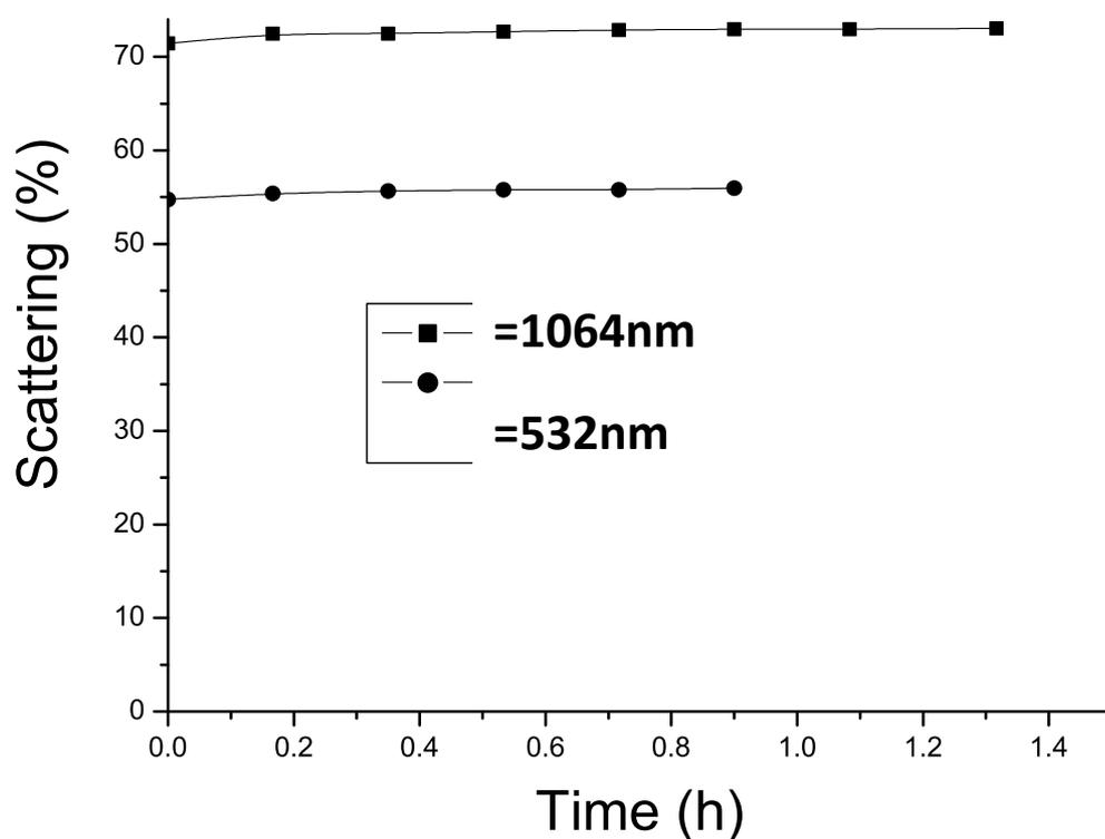
**Figure 4. Time dependence diffused reflection of the tooth @532nm and 1064nm**
